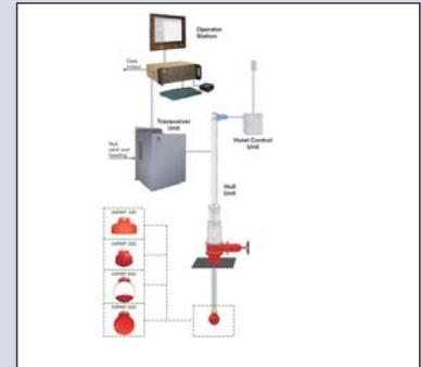
HiPAP was first developed with the focus of using the Super Short Base Line (SSBL) principle, as the market requirement was to try to avoid the Long Base Line (LBL) principle in deep water accurate seabed survey applications. The main advantage of the SSBL principle is that it only requires installation of one vessel-mounted transducer and one subsea transponder.
