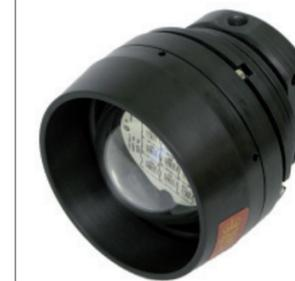
Kongsberg Maritime offers a robust general-purpose white LED lamp for underwater ROV inspection (the model OE11-150). The lamp has a total luminous output of 2460 Lumens, providing an illumination of 800 Lux at a distance of 1m in water.
