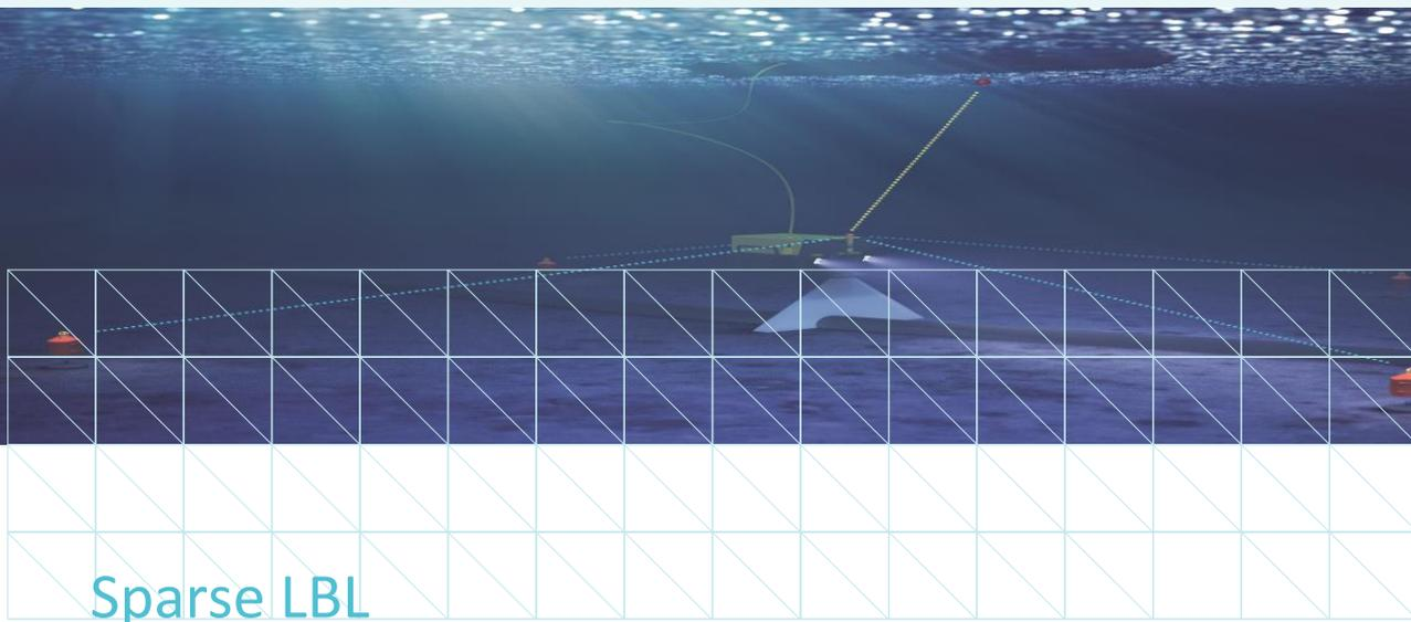
Sparse LBL enables LBL positioning of an ROV using only two cNODE seabed transponders. This function can be combined with HAIN.
