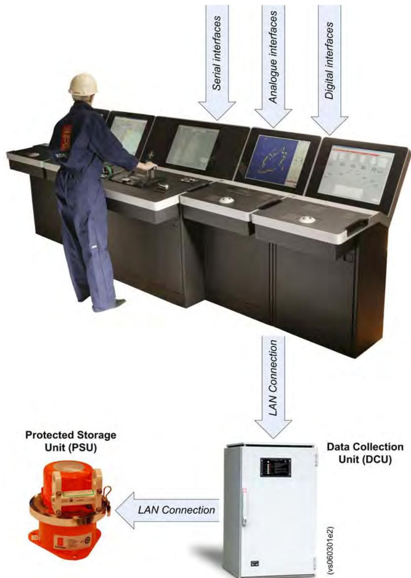
The other extreme is illustrated by the figure below, where none of the systems providing data are supplied by Kongsberg Maritime. In this case each individual data source must be identified, with physical connection points, data formats, estimated data quality etc.
