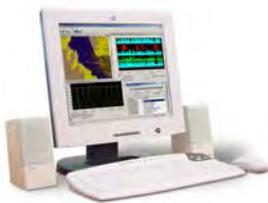
The Replay and Evaluation Unit (REU) is used to replay and evaluate previously recorded time synchronized voyage data.
