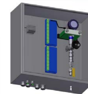
Figure 7: CTU and pressure transmitter cabinet installation
