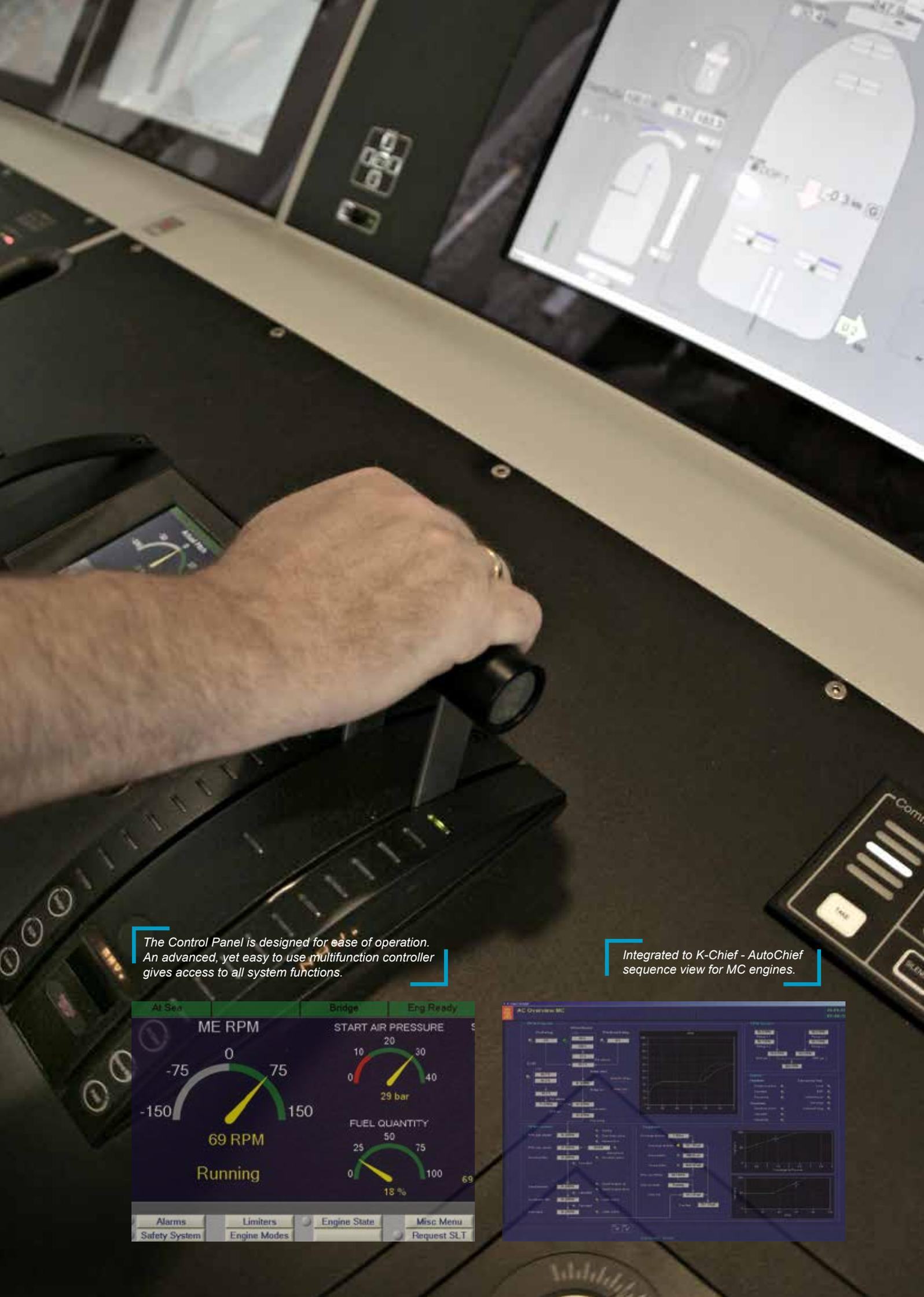
The Control Panel is designed for ease of operation. An advanced, yet easy to use multifunction controller gives access to all system functions.
