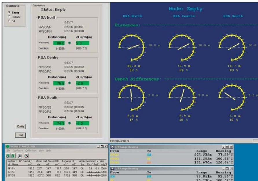
TOTAL Exploration & Production Angola has recently equipped the GIRASSOL FPSO (Block 17, Offshore Angola) with a Riser Tower Monitoring System. The aim of such a system is to provide real time positions of the towers and activate an alarm in case of unusual movement. The three 1300-meter-high riser towers, located 200m away from the barge are mounted with MPT319/DT transponders at the top, 50m below the surface.
