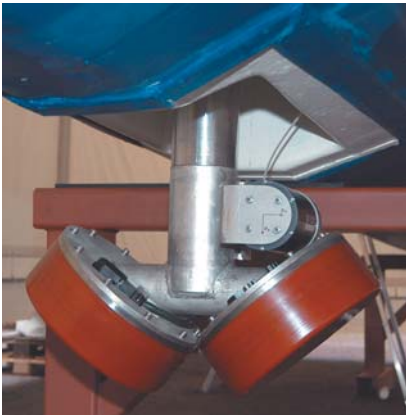
EM 3000 D sonar heads on hoisting arrangement
