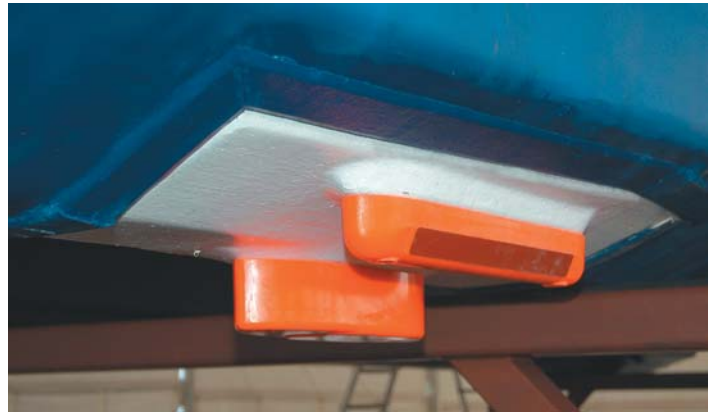
EA 400 38/200 and 120 kHz sidelooking transducers
