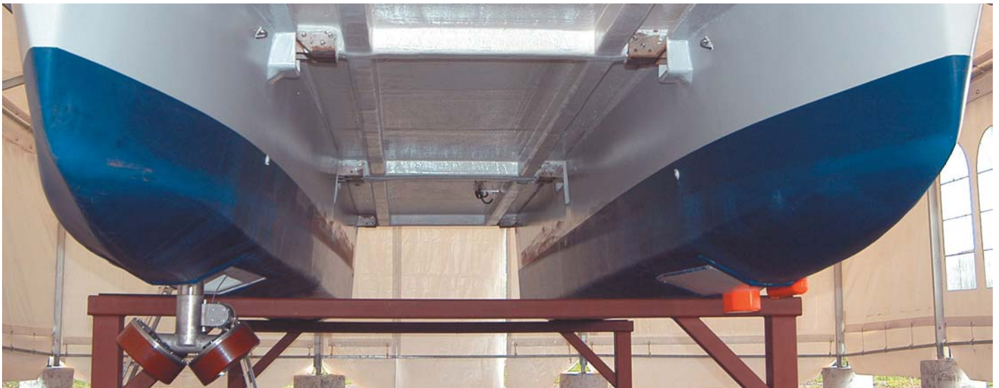
Cassette mounted EM 3000 D, EA 400 38/200 and 120 kHz sidelooking= transducers
