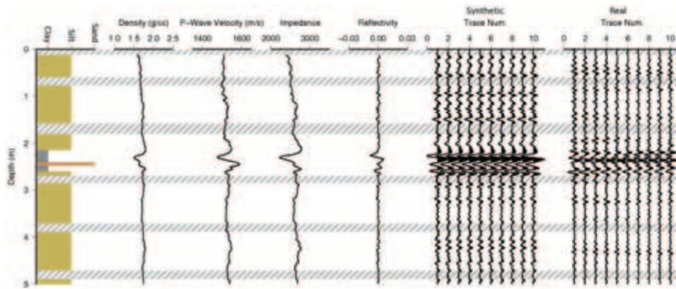
FIGURE 8 Sedimentological, gamma density and P-wave velocity logs from piston core GS-10-163-01, together with impedance, reflectivity and ten synthetic traces calculated using the core logs and theoretical Chirp waveform. For comparison, ten traces from the 3D seismic volume, centred on the core location, are shown. Note the depth values are relative to the top of the core.
