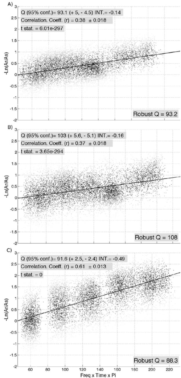
FIGURE 9 Plots of the fjord bed and subsurface reflection amplitude ratios against frequency multiplied by time and Pi using 7000 traces for: the top event bed (A); base event bed (B); and a deeper reflection (C). The gradients of these data are used to estimate robust  $Q$ -factors for the overlying sediments. The grey scale indicates the statistical weight of a data point when calculating robust regression, darker colours representing a stronger contribution (Pinson *et al.* 2008).
