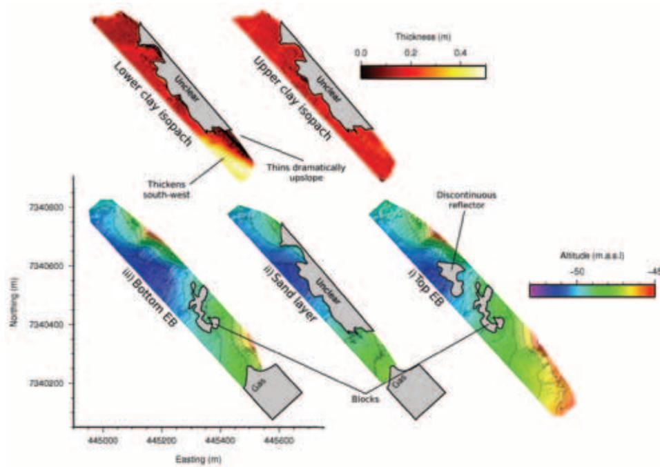
FIGURE 6 Surface maps as interpreted throughout the decimetre-resolution 3D seismic volume for (i) top reflection, (ii) sandy layer and (iii) base reflection of the event bed, together with isopach maps for upper and lower facies, which are representative of the morphology for upper and lower clay-rich layers. Areas of blanking by consolidated slide blocks and gas, together with deformation of top reflection are identified.
