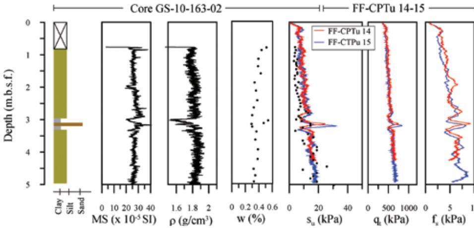
FIGURE 7 Sedimentological, magnetic susceptibility (MS), gamma density ( $r$ ) and water content ( $w$ ) core logs from piston core GS-10-163-02, together with undrained shear strength ( $s_u$ ), total corrected cone resistance ( $q_c$ ) and sleeve friction ( $f_s$ ) from two coincident FF-CPTU profiles (FF-CPTU 14 and 15).
