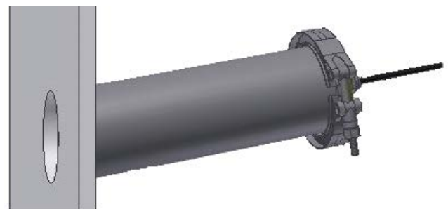
Figure 2. GL-10 welded installation
