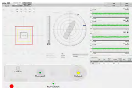
The VMM main view giving an overview of the vessel motion and sensor status.
