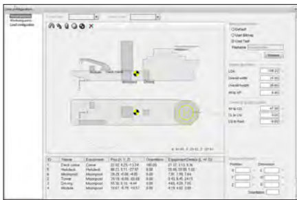
Shows the vessel configuration menu for input and location of the different equipment and monitoring points.
