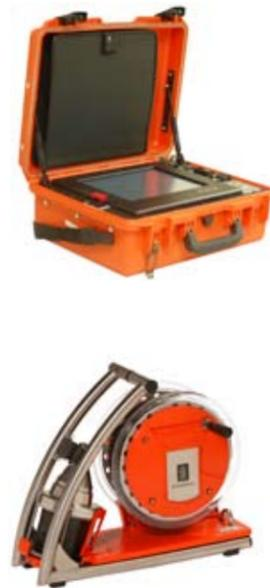
The type approved acoustic control system (ACS) is designed for acoustic control of blow out preventor (BOP) and other subsea production units requiring a control system. Two major subsystems build up the system: The surface part and the subsea part depth rated to 4000m. Each of these two subsystems has transceivers connected to acoustic transducers. The total system is designed based on the principle of full dual redundancy – “two of everything”.
