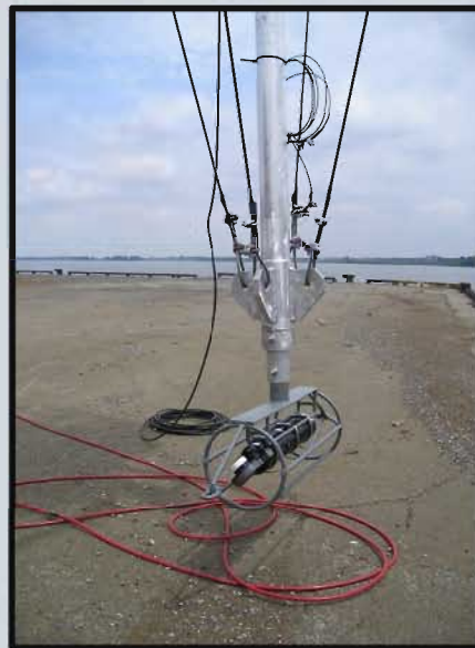
Single RTK GPS antenna is now replaced with a dual antenna unit.
