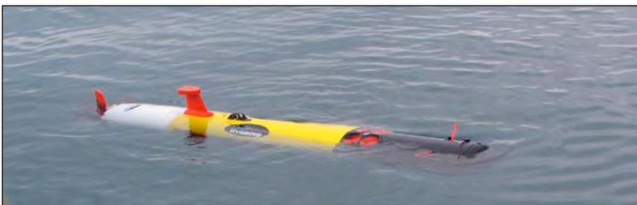
Hydroid will now offer the integration of Kongsberg Maritime's High Precision Acoustic Positioning (HiPAP) system into its family of REMUS AUVs. HiPAP technology will provide REMUS users a faster, more accurate way to obtain an AUV's exact position and to update the vehicle's navigation system.
