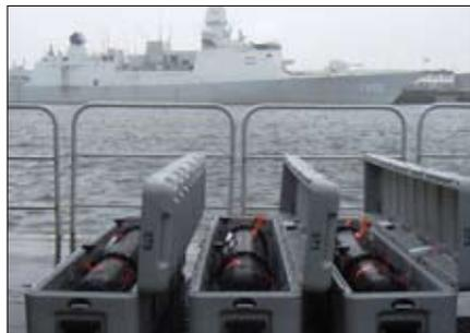
The acquisition also includes upgrades to the RNLN's current fleet of two REMUS 100 vehicles with Marine Sonics' latest generation dual frequency 900/1800 kHz side scan sonars and Kearfott Inertial Navigation as well as training, spares and routine factory maintenance. The current REMUS 100 vehicles have been in operation with the RNLN since February 2005 and have provided a reliable and proven capability for underwater search and survey operations.
