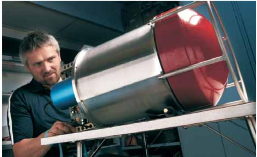
repeatability and high reliability, the HiPAP 100 system is the multi-purpose acoustic positioning system for ultra deep water operations.
