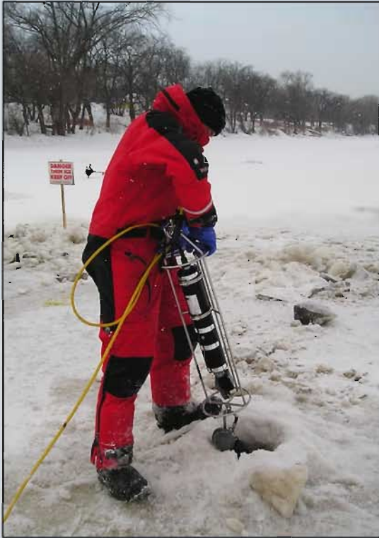
Winnipeg Police officer deploying the cage-mounted sonar head into an augered hole at -26°C (-15°F).
