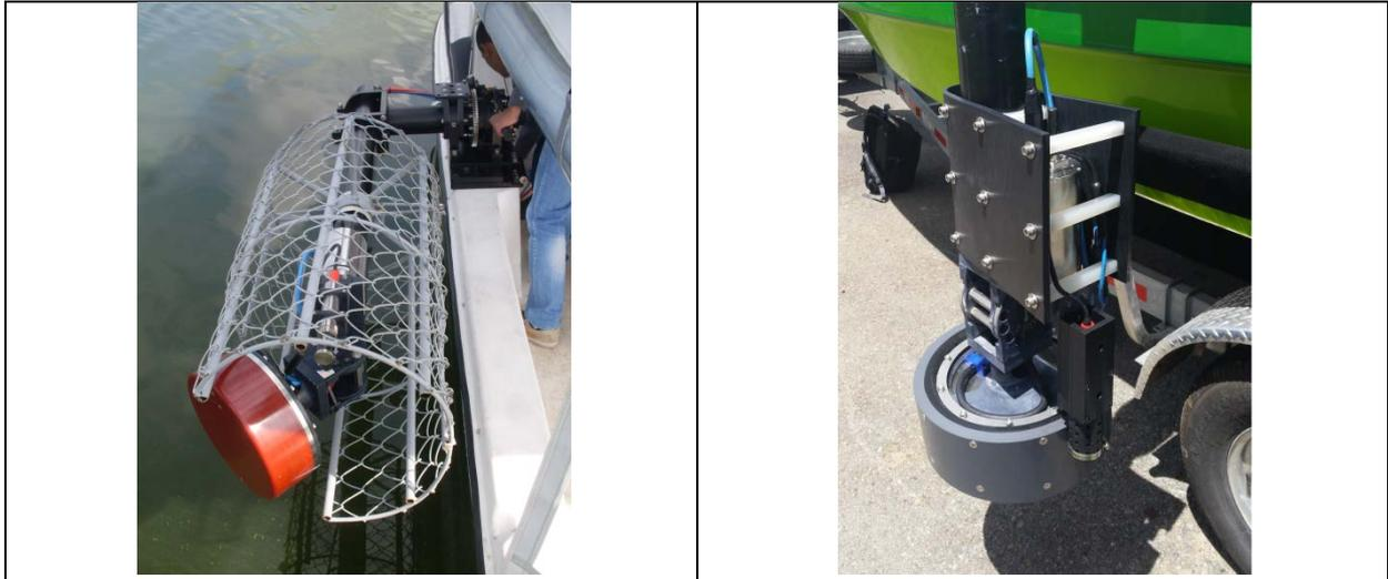
*Several protection devices were designed to protect the Sonar Head, MRU-5 and SV Probe.*
