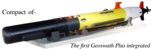
*The first Geoswath Plus integrated with a man-portable REMUS AUV*
