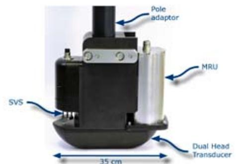
*The compact wet-end for over-the-side mounting holds the dual head transducer together with the ancillary sensor. It can be pre-calibrated and weights as little as 17 kg.*
