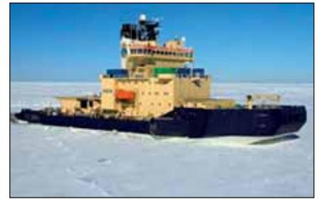
is 1.9 m level ice at 3 knots (5.5 km/h), 8 metre core ice.
