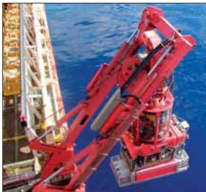
*Triton XLS ROV: Canyon Offshore Triton XLS02 ROV with an attached seabed node skid*
