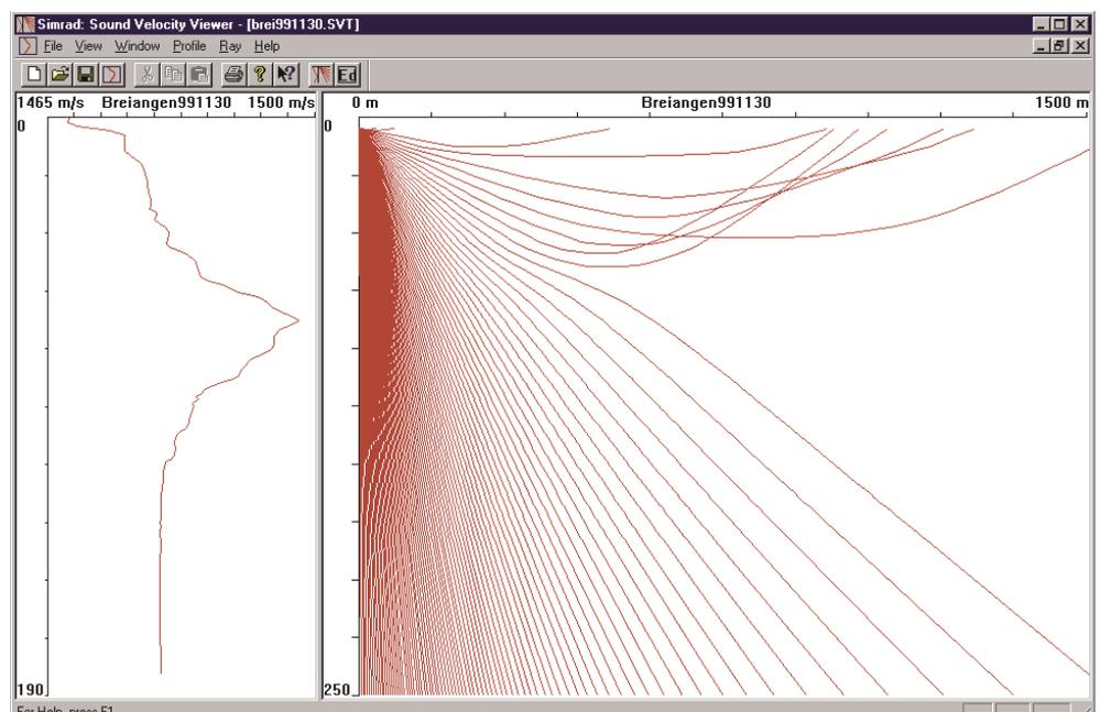
The function is not only error correcting, it also gives the operator a tool to see the limitations of the nature, as well as it can give the answer to a range problem. Wrong sound velocity input gives error in absolute accuracy, but influences very little in relative position changes and stability.
