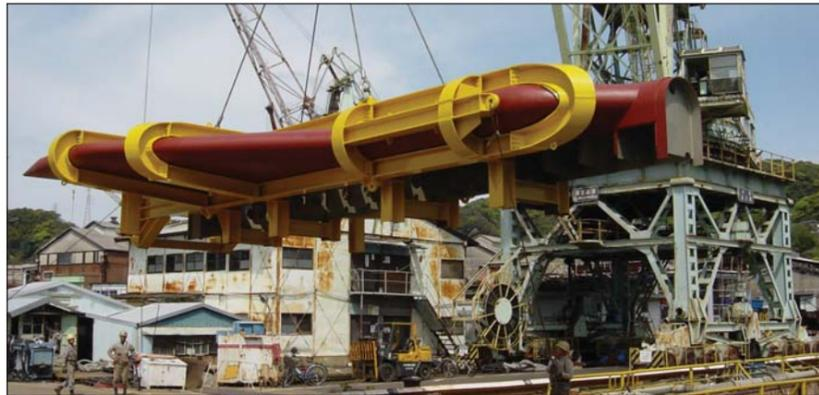
All of the acoustic sensors were installed on a newly designed "gondola" measuring 8 meters across (athwartships) and over 14 meters in length.
