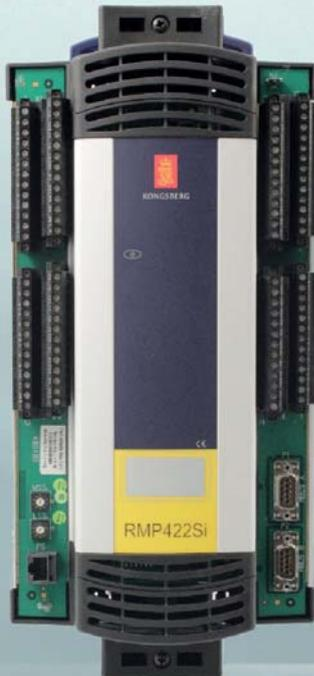
RMP422Si is an RBUS IO module with 32 HART enabled analog input field channels for use in safety applications. The input channels are individually software configurable for the appropriate signal type and parameters. The module has extended loop monitoring including current leak detection on each channel. The module is certified for use in hazardous area zone 2.
