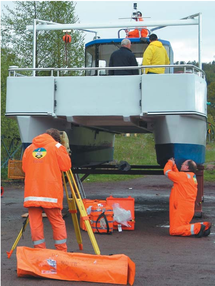
Alignment of the survey equipment
