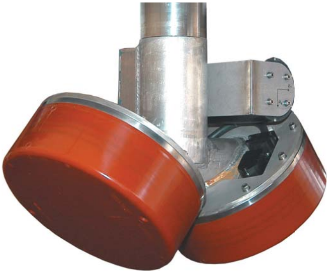
EM 3000 D specially designed hull unit for ConCat
