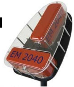
The basic EM 2040 consists of four units; transmit transducer, receive transducer, processing unit and an operator workstation. The EM 2040 has a standard depth rating of 6000 m and is fully prepared for installation and operation on subsea vehicles such as AUVs and ROVs.
