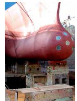
The R/V Melville, 97 m long with a displacement of almost 3000 tons, is one of the largest oceanographic research vessels in the U.S. academic (UNOLS) fleet. The photos above were taken during the recent EM 120 installation in Japan. (No – the windows in the bulbous bow are not there to provide the multibeam operator with a scenic view!)
