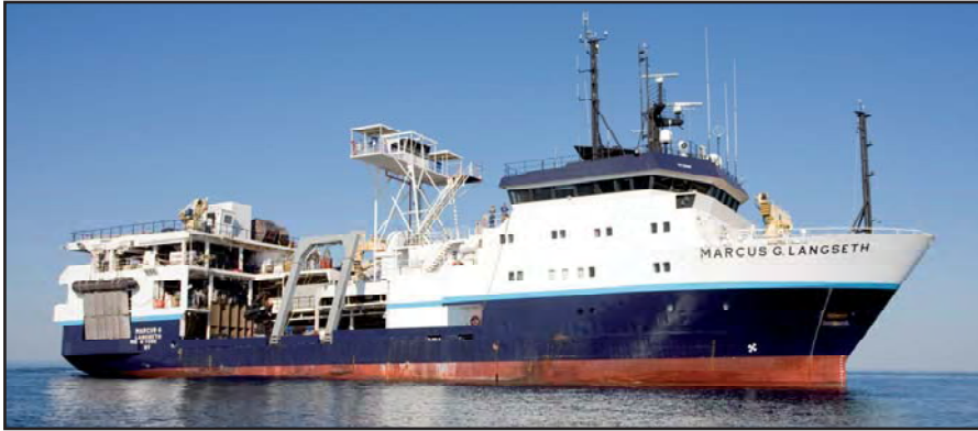
The R/V Marcus G. Langseth is a 71.5 m long, 2578 ton research vessel owned by the National Science Foundation and operated by Lamont-Doherty Earth Observatory of Columbia University.
