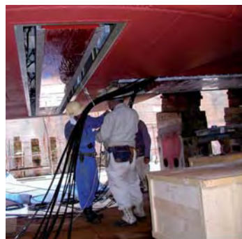
The R/V Melville, 97 m long with a displacement of almost 3000 tons, is one of the largest oceanographic research vessels in the U.S. academic (UNOLS) fleet. The photos above were taken during the recent EM 120 installation in Japan. (No – the windows in the bulbous bow are not there to provide the multibeam operator with a scenic view!)
