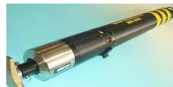
Transponders generate an acoustic pulse in response to the acoustic interrogation signal from the transducer. The acoustic response can be configured to provide a depth telemetry signal. One transponder must be fitted to each underwater unit that is required to be tracked.
