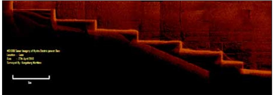
A mosaic image showing high resolution MS1000 Sonar scans of a 55m section of the dam wall. Water visibility is less than 0.2m in the dam.
