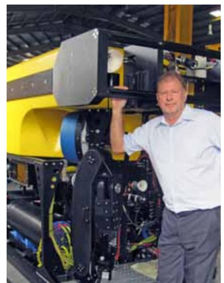
*Eastar Offshore Pte Ltd Operations manager Stuart Raines with the Deep Swift 2 ROV. This is a 3000m depth rated, 175HP workclass ROV.*
