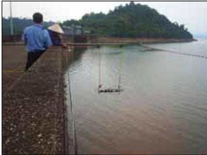
The MS1000 high resolution sonar is lowered into the dam.
